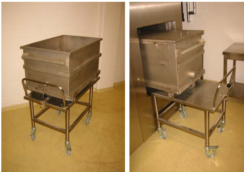
Abb. 28 Loading device of a steam disinfection plant
