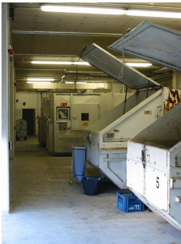
Abb. 8 Central waste storage hall with transportable compactors for general HCW
