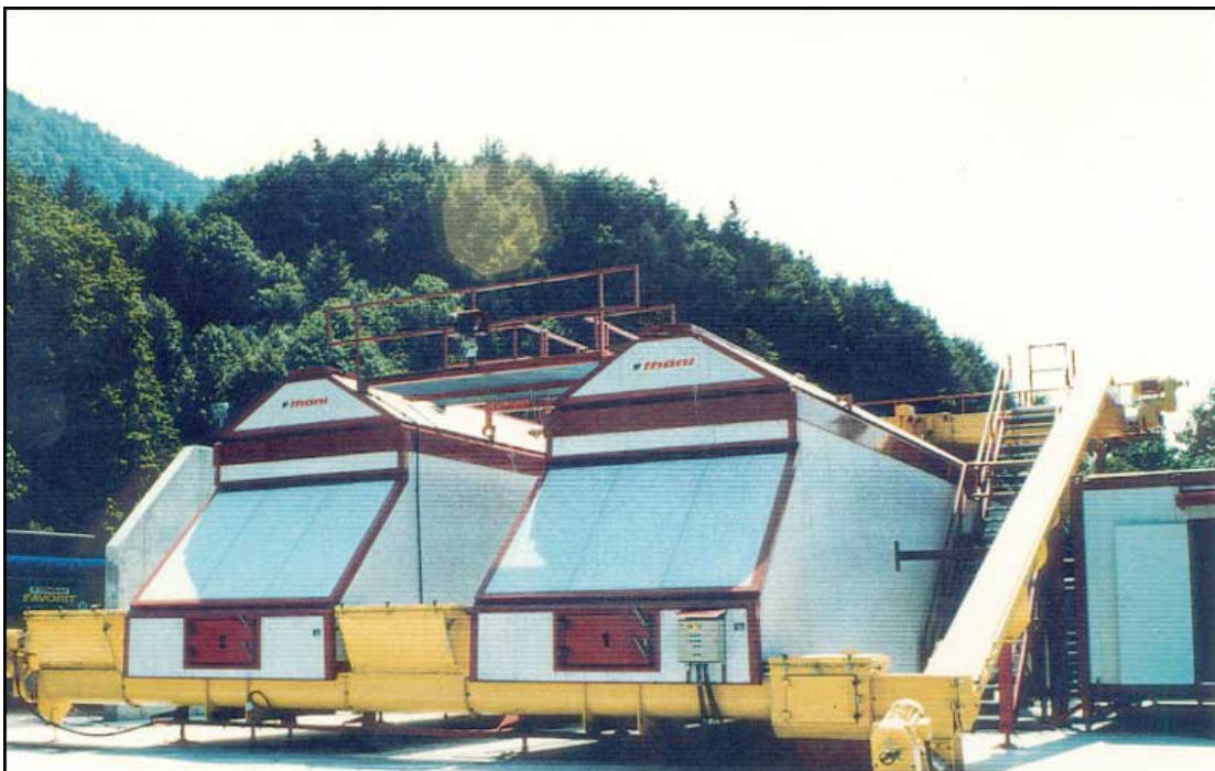
Fig. 5.15: Container Composting System Thöni (Photo: Thöni)
