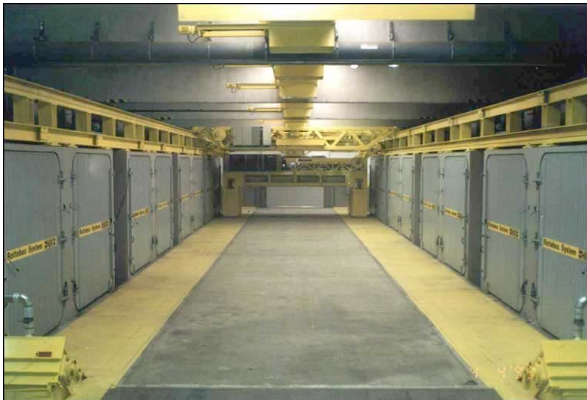
Fig. 5.13: Box Composting System Herhof (Photo: Herhof)
