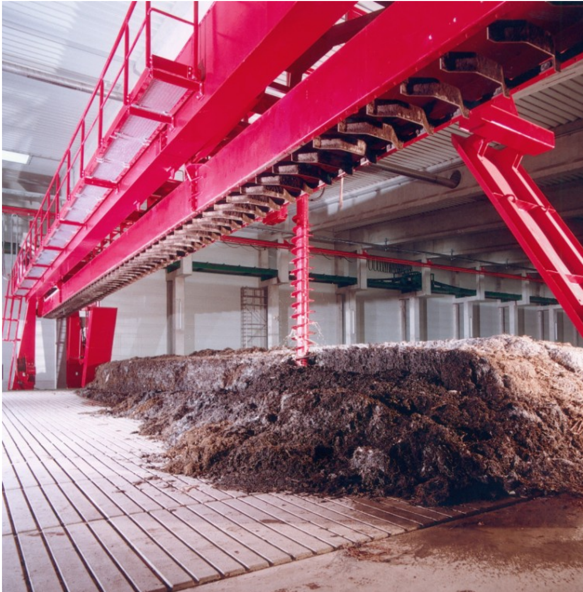
Fig. 5.23: Windrow Composting System Thyssen „Dynacomp“ (Foto: Thyssen)
