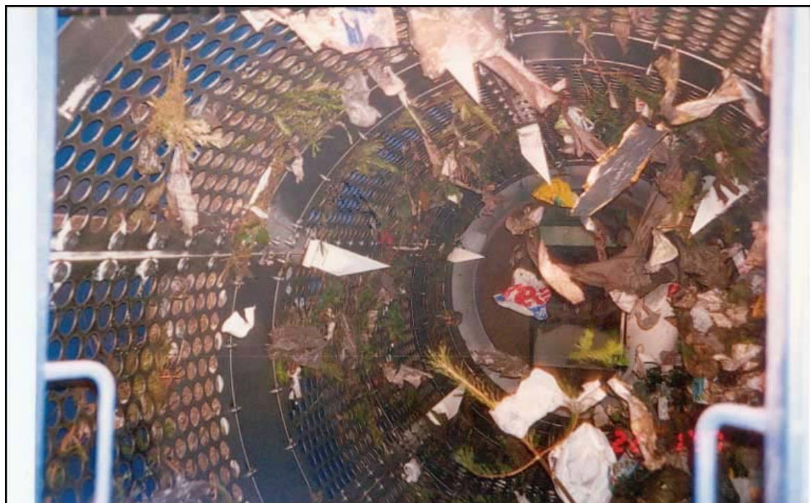
Fig. 5.6: View into the Drum Screen (Photo: Ingenieurgesellschaft Abfall)
